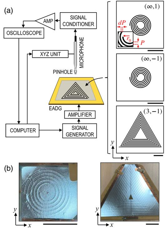
FIG. 2. (a) Sketch of the experimental setup involving 2D structured electroactive diffraction gratings (EADG). (b) Top view of the fabricated acoustic sources corresponding to the Bessel beam with  $(N, \ell) = (\infty, 1)$  and three-wave interference  $(N, \ell) = (3, -1)$ . Scale bars: 5 cm.
