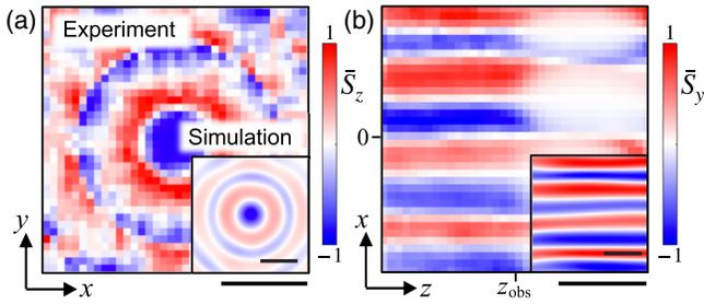
FIG. 7. Experimentally retrieved and numerically calculated (insets) distributions of the longitudinal  $z$  and transverse  $y$  components of the normalized spin density  $\bar{\mathbf{S}}$  in the transverse  $(x, y)$  (at  $z = z_{\text{obs}}$ ) and meridional  $(z, x)$  (at  $y = 0$ ) cross sections of the Bessel beam with  $\ell = -1$ . Flipping the sign of  $\ell$  flips the sign of  $\bar{S}_z$  (see Supplemental Material, Sec. I [46]) but not  $\bar{S}_y$  [5]. Scale bars:  $\lambda$ .
