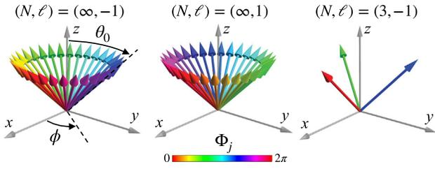
FIG. 1. Wave vectors of  $N$  interfering plane waves, Eqs. (1) and (2), evenly distributed over the cone with the polar angle  $\theta_0 = \pi/4$  and having relative vortex phases  $\Phi_j = \ell\phi$  (color coded). The three cases shown here correspond to the Bessel beams with  $\ell = \pm 1$  and a three-wave interference with  $\ell = -1$ .
