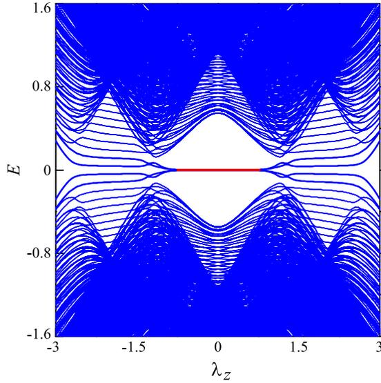
FIG. 3. BdG energy spectrum with open boundary conditions in the  $x$  and  $y$  directions as a function of  $\lambda_z$ . The sample size is  $20 \times 20$ . The red line corresponds to eightfold-degenerate MCSs, which exist only for finite amplitudes of the exchange field. The parameters are chosen to be  $m_0 = -0.8$ ,  $\lambda_{\text{so}} = 1$ ,  $m_x = m_y = 1$ ,  $\mu = 0$ , and  $\Delta_1 = 0.5$ .
