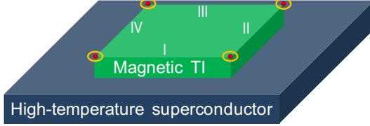
FIG. 1. Schematic view showing a magnetic TI approximated by a high-temperature superconductor. The Majorana bound states are located at the four corners of the green square sample. I, II, III, and IV label the four edges of the lattice.
