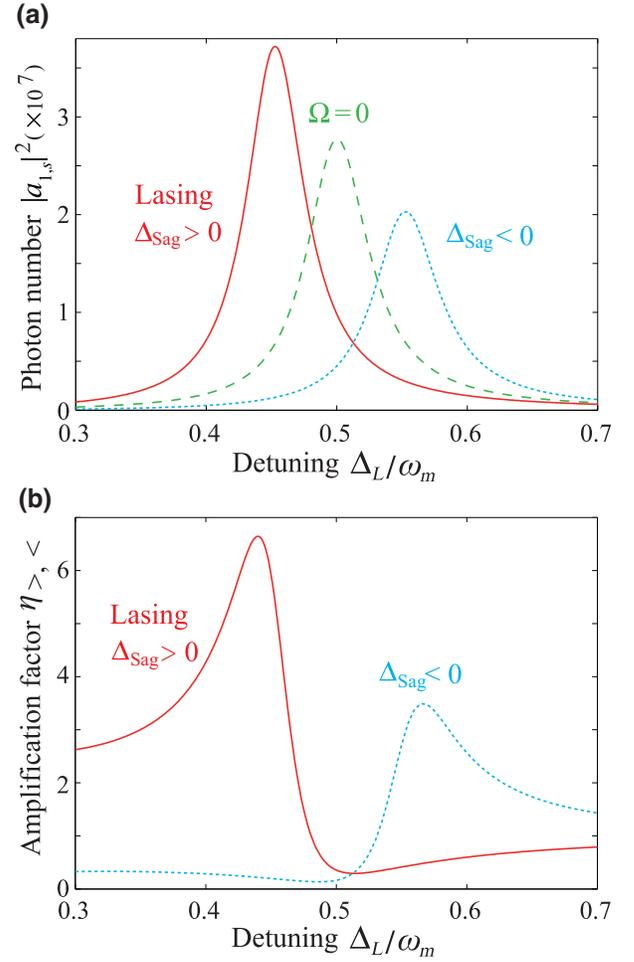
FIG. 2. (a) The steady-state photon number  $|a_{1,s}|^2$  as a function of the optical detuning  $\Delta_L$ . The dependence of  $|a_{1,s}|^2$  on the spinning speed  $\Omega$  is clearly seen. (b) The mechanical displacement amplification factor  $\eta$  versus  $\Delta_L$ . Parameters are chosen as  $\Omega = 6$  kHz,  $J/\omega_m = 0.5$ , and  $P_{\text{in}} = 10$   $\mu$ W.
