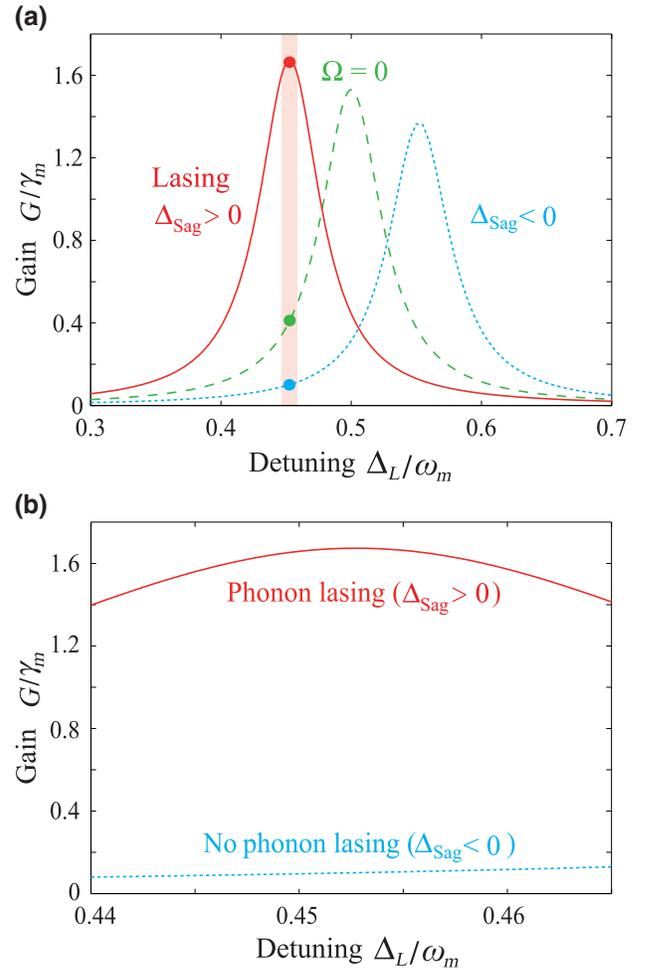
FIG. 3. (a,b) The scaled mechanical gain  $G/\gamma_m$  as a function of the optical detuning  $\Delta_L$ . Phonon lasing can be generated (red curve) or prohibited (blue curve) for different rotation directions, indicating that acoustic nonreciprocity can be achieved, as shown in (b). The thick points in the vertical pink band in (a) correspond to two different driving directions at  $\Delta_L/\omega_m = 0.45$ . The other parameters are the same as those in Fig. 2.
