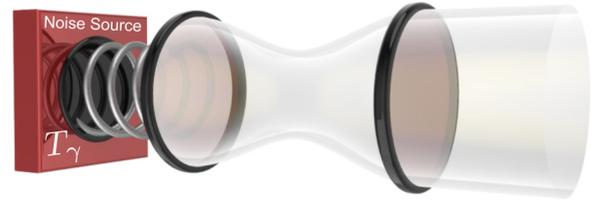
FIG. 1. Schematic of a generic optomechanical system. One of the mirrors of the optical cavity is coupled to a noise source with effective temperature  $T_\gamma$  and can vibrate at frequency  $\omega_m$ . This system can generate Casimir photon pairs.
