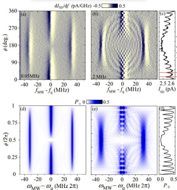
Comparison of the measured peak currents (top) and the calculated excitation probabilities (bottom) showed a perfect match for the device in the incoherent regime (left) and coherent regime where the function becomes a superposition of heat engine and refrigerator operation (right). Credit: Physical Review Letters
