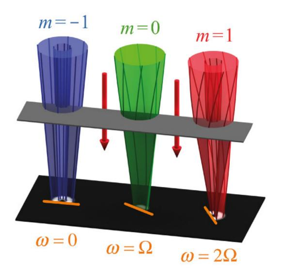
Electrons moving in a magnetic field rotate at three frequencies—0, the Larmor frequency ( $\Omega$ ), and the cyclotron frequency ( $2\Omega$ )—depending on the quantum number describing their angular momentum (m).
