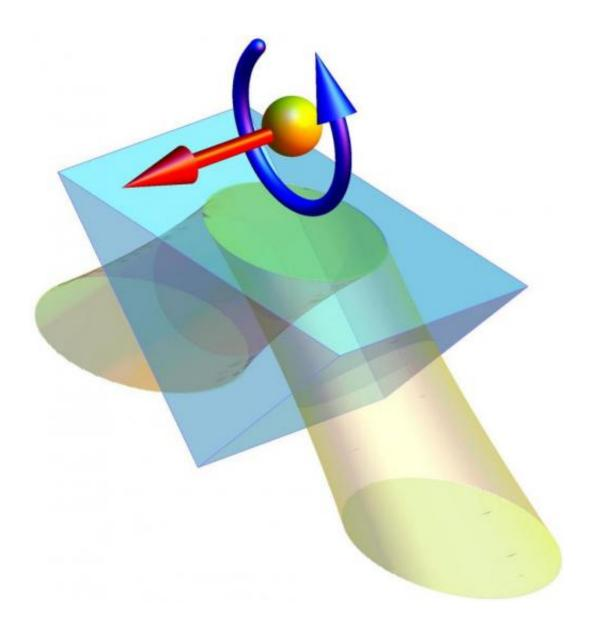
Transverse force (red) and torque (blue) exerted on a particle (yellow sphere) in an evanescent field generated by total internal reflection in a glass prism. Credit: © 2014 Konstantin Bliokh, RIKEN Interdisciplinary Theoretical Science Research Group
