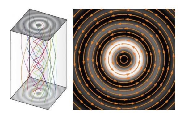
Reconstruction of photon trajectories (left) from the measured transverse momentum of light (right) in a vortex beam. Credit: Reproduced from Ref. 1 and licensed under CC by 3.0 at dx.doi.org/10.1088/1367-2630/15/7/073022. © 2013 K. Bliokh et al.
