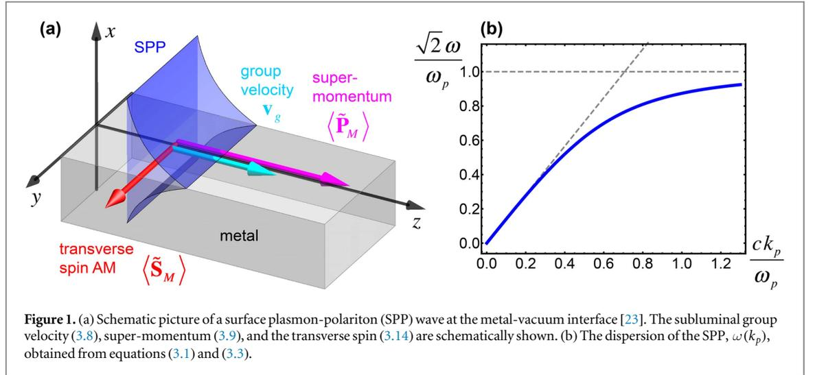
**Figure 1.** (a) Schematic picture of a surface plasmon-polariton (SPP) wave at the metal-vacuum interface [23]. The subluminal group velocity (3.8), super-momentum (3.9), and the transverse spin (3.14) are schematically shown. (b) The dispersion of the SPP,  $\omega(k_p)$ , obtained from equations (3.1) and (3.3).
