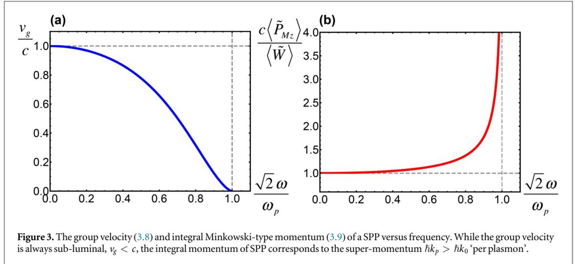
**Figure 3.** The group velocity (3.8) and integral Minkowski-type momentum (3.9) of a SPP versus frequency. While the group velocity is always sub-luminal,  $v_g < c$ , the integral momentum of SPP corresponds to the super-momentum  $\hbar k_p > \hbar k_0$  ‘per plasmon’.
