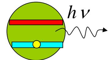
Finally, the qubit is in its ground state and one photon is emitted.
