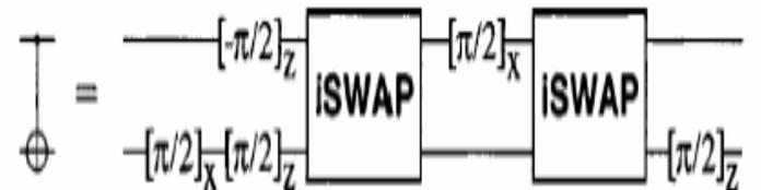
Quantum tomography can be implemented via an ISWAP gate, even if only one qubit measurement can be performed at a time.
