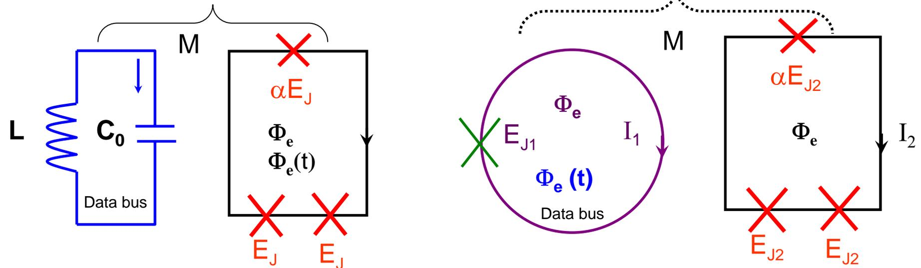
The circuit with an LC data bus models the Delft circuit in Nature (2004), which does not work at the optimal point for a TDMF to control the coupling between the qubit and the data bus.
