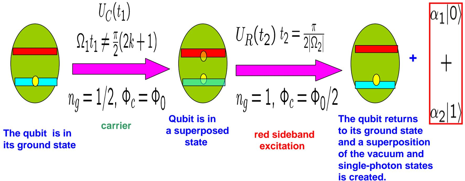
When the red sideband excitation satisfies the condition  $t_2 = \pi/2|\Omega_2|$ , it creates a superposition of the vacuum and single photon states.
