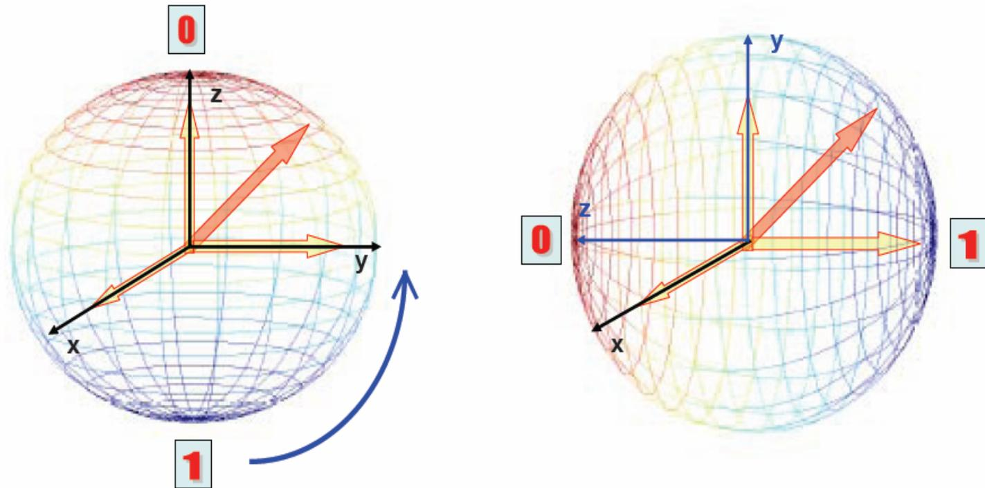
This rotation can be realized by setting  $\Phi_x = 0$  and  $n_c = \frac{1}{2}$  with an evolution time  $t_x = \frac{\hbar\pi}{4E_J^0}$ .
