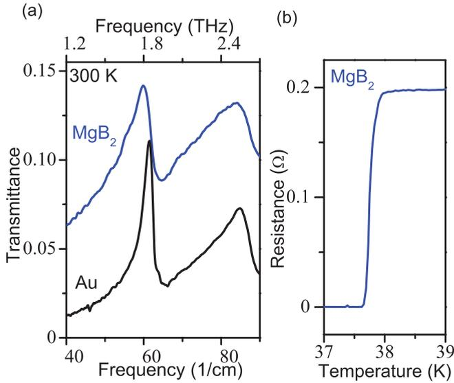
FIG. 1. (Color online) Experimental results for a  $\text{MgB}_2$  film and a Au film with arrays of subwavelength holes. (a) Transmission spectra for both films at 300 K. (b) Resistance vs temperature for the  $\text{MgB}_2$  film.
