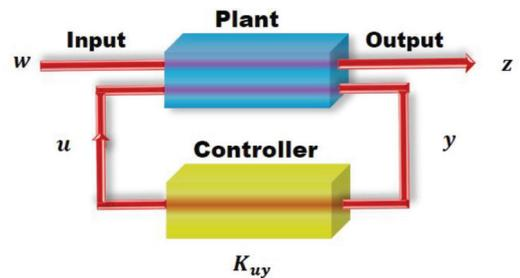
FIG. 6. (Color online) Diagram of the input-output model of the coherent feedback system in Fig. 5(b).
