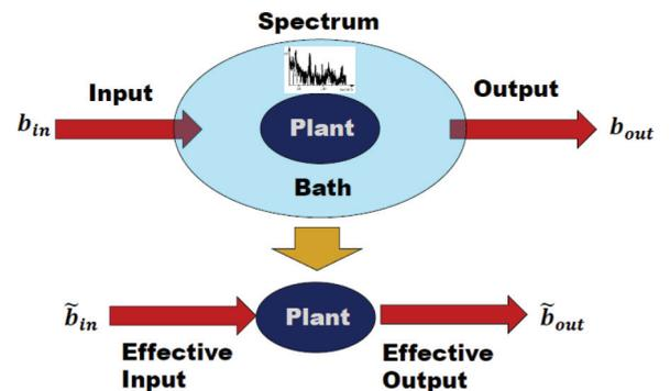
FIG. 3. (Color online) Effective non-Markovian input-output model obtained from a larger Markovian input-output system in which the Markovian input and output fields interact with an intermediate bath, which is then coupled to the plant we consider.
