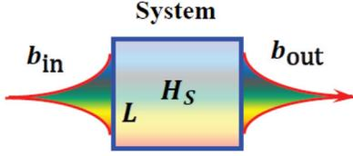
FIG. 2. (Color online) Schematic diagram of the non-Markovian input-output system. The input field is dispersed when it interacts with the system, and the modes with different frequencies in the input field are coupled to the system with different coupling strengths.
