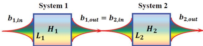
FIG. 8. (Color online) Schematic diagram of the non-Markovian quantum cascade system. The output from the first subsystem is fed into the input of the second subsystem.
