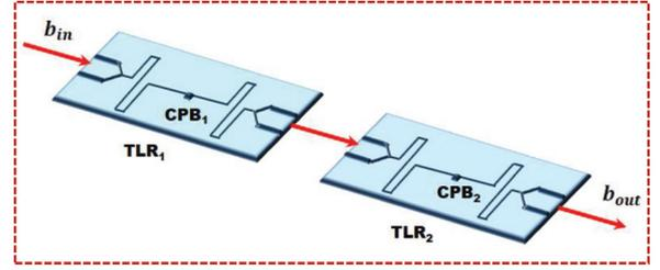
FIG. 9. (Color online) Schematic diagrams of two cascade-connected Cooper-pair box and transmission-line resonator (CPB-TLR) input-output systems.
