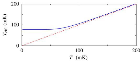
FIG. 3 (color online). The effective noise temperature,  $T_{\text{eff}}$ , in the output field of the CPW, versus the input-field temperature,  $T$ , at  $\omega_d/2$ , half the driving frequency. The (red) dashed line shows the result for purely thermal radiation, and the (blue) solid line for both thermal and quantum radiation. For low enough temperatures, the quantum radiation is significantly larger than the thermal noise level. Here, we used the same parameters as in Fig. 2.
