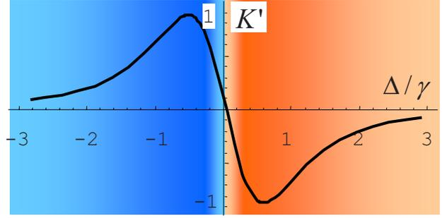
FIG. 3. (Color online) The effective elastic constant  $K'$  (arbitrary units) versus the detuning  $\Delta = \omega_{rf} - \omega_{a0}$  (scaled by  $\gamma$ ). When  $\omega_{rf} < \omega_{a0}$ , the beam can be cooled. Here, the region  $\Delta > 0$  ( $\Delta < 0$ ) is shaded by the red (blue) color, representing the heating (cooling) of the beam, respectively.
