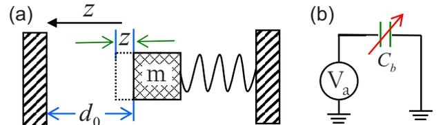
FIG. 2. (Color online) (a) Schematics of the beam (mass and spring) capacitively coupled to a conductor and (b) its equivalent circuit. The charging energy of the beam is determined by the voltage  $V_a$  and variable capacitor  $C_b$  between the beam and the 1D transmission line.
