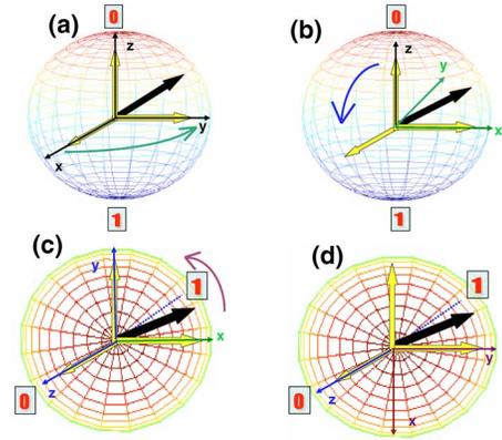
FIG. 2. (Color online) The Bloch vector is the same as Fig. 1. A  $-\pi/2$  rotation of the qubit along the  $y$  direction is equivalently realized by the rotation  $\pi/2$  of the measuring instrument along the  $z$  direction [from (a) to (b)], then a  $\pi/2$  rotation along the  $x$  direction [from (b) to (c)], and a  $3\pi/2$  rotation along  $z$  direction [from (c) to (d)].
