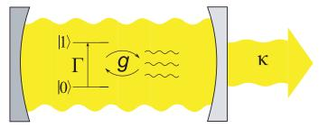
**Figure 1.** Schematic diagram of a two-level atom interacting with a cavity mode. The coupling strength for the exchange of excitations between the atom and the cavity is g. The atom is biased such that it experiences 'inverted relaxation' from the ground to the excited state, with rate  $\Gamma$ . The loss rate of photons out of the cavity is  $\kappa$ .
