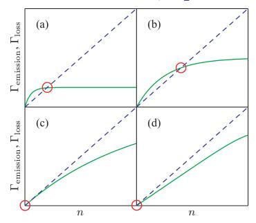
**Figure 2.** Schematic plot of the photon emission rate  $\Gamma_{\text{emission}}$  (green solid line) and the photon loss rate  $\Gamma_{\text{loss}}$  (blue dashed line) as functions of the photon number in the cavity *n*. The intersection point (red circle) determines the value of *n* in the photon-number probability distribution with the highest probability. Going from (a) to (d),  $\Gamma$  is increased, whereas  $\kappa$  is kept fixed.
