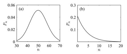
**Figure 4.** Occupation probability as a function of photon number in the cavity for a point in the lasing regime (a;  $\Gamma \kappa / (4g^2) = 0.5$ ) and one in the thermal regime (b;  $\Gamma \kappa / (4g^2) = 1.25$ ). The system parameters are given in figure 3. The curve in (a) is fitted very well by a Gaussian function, and the curve in (b) is fitted very well by a Boltzmann thermal-distribution function.
