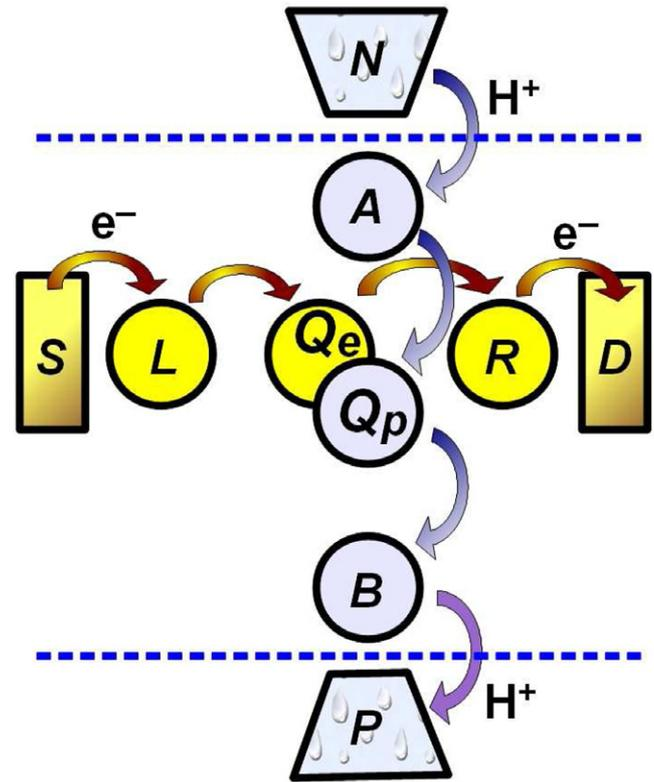
**Figure 1.** Schematic diagram of the static proton pump. The electron-transport chain starts at the source (S) lead. Thereafter, high energy electrons,  $e^-$ , tunnel *energetically downhill* (through the yellow path) to the sites L,  $Q_e$ , R and, finally, to the drain (D). Low energy protons,  $H^+$ , move *energetically uphill* (in blue) from the N-side of the membrane to the sites A,  $Q_p$ , B and, eventually, reach the P-side of the membrane.
