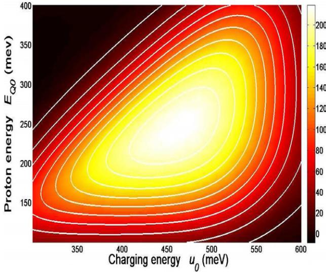
**Figure 5.** Dependence of the proton current (the number of protons pumped across the membrane per one  $\mu\text{s}$ , see the color bar on the right side) on the charging energy  $u_0$ , and on the energy  $E_{Q0}$  of the central proton site for  $V_e = 600$  meV,  $V_p = 150$  meV, and  $T = 298$  K.
