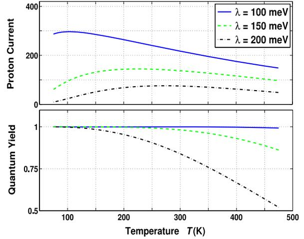
**Figure 4.** Proton current (the number of protons translocated across the membrane per 1  $\mu$ s) and QY versus temperature for the electron voltage  $V_e = 600$  meV, transmembrane proton voltage  $V_p = 150$  meV, and three different reorganization energies:  $\lambda = 100, 150,$  and  $200$  meV. The proton current and QY both decrease for increasing  $\lambda$ .
