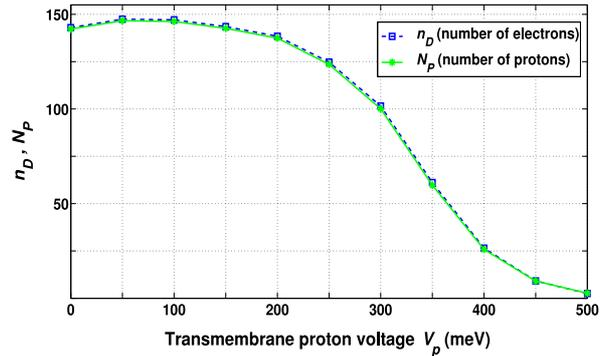
**Figure 7.** Numbers of electrons,  $n_D$ , and protons,  $N_P$ , translocated across the membrane in one millisecond, versus the transmembrane proton voltage  $V_p$  at room temperature,  $T = 298$  K, and at  $(\mu_S - \mu_D) = 650$  meV. Clearly, it is much harder to transfer protons against the higher transmembrane voltages.
