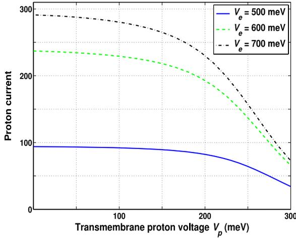
**Figure 3.** Proton current versus transmembrane voltage  $V_p$  at room temperature,  $T = 298$  K, and three different electron potentials:  $V_e = 500, 600,$  and  $700$  meV. The proton current is almost constant for low values of  $V_p$ , and decreases for increasing  $V_p$ .
