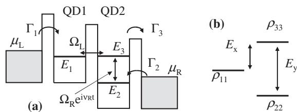
**Fig. 1.** (a) A three-level system in double QDs (DQDs). A bias voltage is applied between the left and right electrodes. (b) A density matrix for the three level. We define  $E_x \equiv E_3 - E_1$  and the detuning  $E_y \equiv E_3 - E_2 - v_R$ . The dark state is a state with  $\rho_{33} = 0$ .
