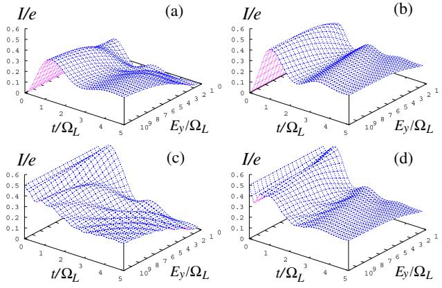
**Fig. 5.** (Color online) Time-dependent current as a function of  $E_y$  starting from  $|1\rangle$  for (a) and (b),  $(|1\rangle + |2\rangle)/2$  for (c) and (d).  $\Gamma_1/\Omega_L = \Gamma_2/\Omega_L = \Gamma_3/\Omega_L = 1$ ,  $\gamma_0/\Omega_L = 1$ , (a, c)  $t_0/\Omega_L = 0$  and  $\gamma_{21}/\Omega_L = 0$ . (b, d)  $t_0/\Omega_L = 1$  and  $\gamma_{21}/\Omega_L = 1$ .
