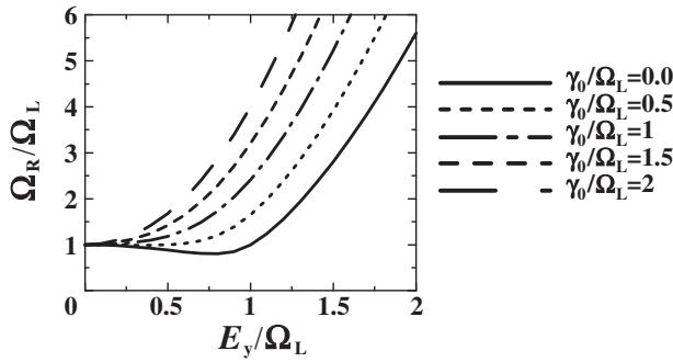
**Fig. 2.** The Rabi frequency  $\Omega_R$  needed for realizing a dark state, as a function of the detuning  $E_y$  and  $\gamma_0$ . Here,  $E_x = 0$ ,  $\gamma_{21} = 0$ ,  $t_0 = 0$ , and  $\Gamma_1 = \Gamma_2 = \Gamma_3$ . These are solutions of  $\rho_{33} = 0$  in eq. (9).
