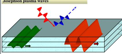
One of the ways to excite surface waves is via externally applied electromagnetic waves on a sample having spatially modulated parameters.
