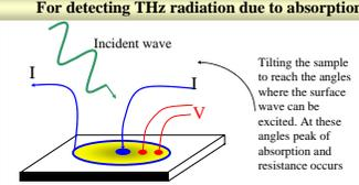
The resonance in the absorption can be observed by measuring the dependence of the surface impedance on the angle  $\theta$ . Alternatively, the peak in absorption produces a temperature increase, resulting in a sharp increase of the DC resistance or even the transition of the sample to the normal state at  $\theta = \theta_0$ .
