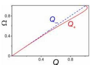
Spectra of two branches "±" of the surface Josephson plasma waves for the parameters  $\alpha = 0.1$  and  $\beta = 1.4$ , standard for Bi2212.
