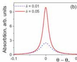
Absorption obtained for different effective dampings
