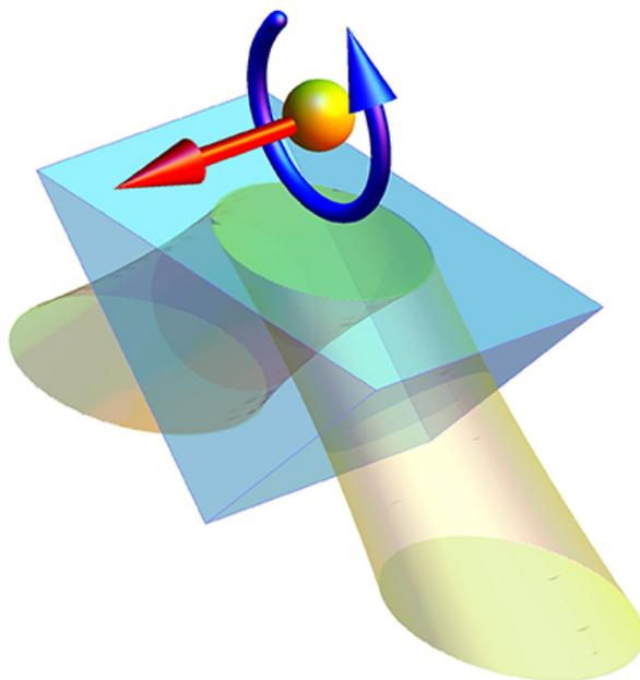
Transverse force and torque on a particle in evanescent field generated from a total internal reflection in a glass prism. These reveal the presence of the transverse momentum and spin in the evanescent wave above the prism.
