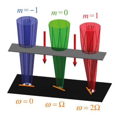
Electrons moving in a magnetic field rotate at three frequencies—0, the Larmor frequency ( $\Omega$ ), and the cyclotron frequency ( $\Omega$ )—depending on the quantum number describing their angular momentum (m).
