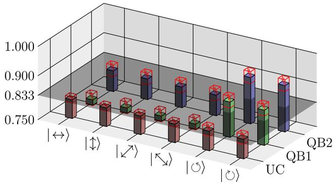
FIG. S2: Single-copy fidelities  $\bar{F}_i$  for the states with different linear and circular polarizations measured during the encoding of our two quantum banknotes 1 and 2 (QB1 for  $\epsilon = 0$  and QB2 for  $\epsilon = 0.4$ ), and the optimal universal cloner (UC for  $\epsilon = 0$ ). The grey surface shows the theoretical fidelity of the universal cloner. The red frames show the error bars of the measured fidelities. This figure can be compared with Figs. 5 and 6 in the main article.
