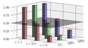
**Fig. 5** Success probabilities of the cloning processes for quantum banknotes 1 and 2 (QB1 and QB2), and optimal universal cloning (UC). The red frames show the error bars of the measured probabilities. The gray surface shows the minimum cloning efficiency needed to output on average more cloned photons than the input photons
