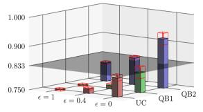
**Fig. 6** Experimentally measured average cloning fidelity  $\overline{F}_i$  for quantum banknotes 1 and 2 (QB1 and QB2), and optimal universal cloning (UC). The red frames show the error bars of the measured probabilities. The verification threshold (gray surface) is set at 0.833, which is the fidelity of the optimal universal cloning process, i.e., the process that ignores any information about g
