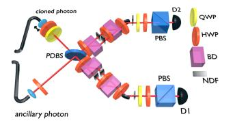
**Fig. 3** Experimental setup for cloning quantum bankotes. Components are labeled as follows: HWP is half-wave plate, QWP is quarter wave-plate, PDBS is polarization dependent-beam splitter, PBS is polarizing beam splitter, BD is beam divider, NDF is neutral density filter, and D is single photon detector. A successful cloning and verification of a qubit from a given sequence is registered as a simultaneous detection event at the two detectors
