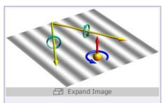
Figure 1: Two interfering plane waves (yellow arrows) exert a force (red) and torque (blue) on a small particle (yellow sphere) perpendicular to the interfering waves.
