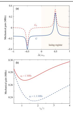
FIG. 2. (a) The mechanical gains  $G_0$  (without defect) and G (with defect) as a function of the optical detuning  $\Delta$ . (b) G as a function of the defect loss  $\gamma_q$ . Here, for simplicity, we use  $\gamma_q/\gamma=1$ ,  $g_d=1$  MHz in (a),  $\Delta=0.5\omega_m$  in (b), and  $J=0.5\omega_m$  and  $P_I=10~\mu{\rm W}$  in both (a) and (b).
