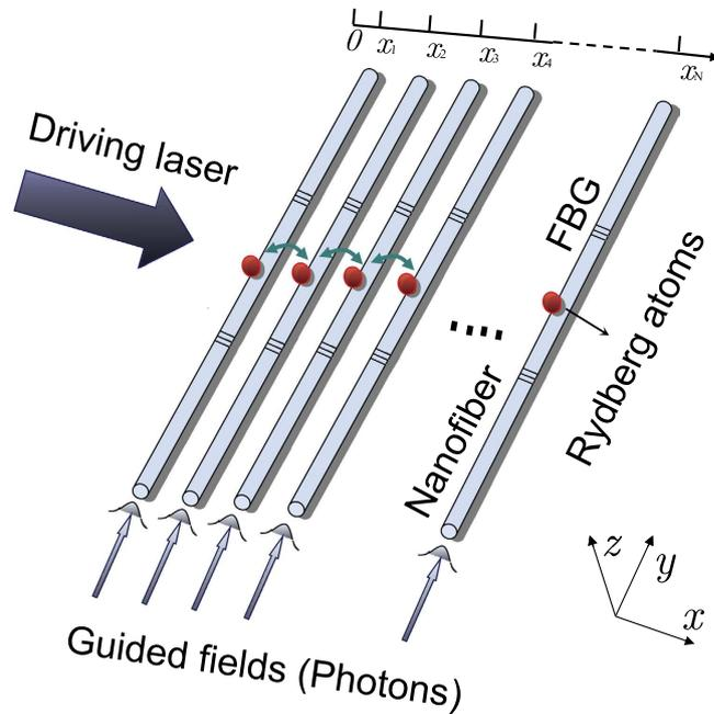
**Figure 1. Schematic diagram of the system studied.** A 1D nanofiber photonic crystal cavity array, with an ensemble of Cs Rydberg atoms (red disks) placed near each nanofiber. Photons can hop between two adjacent cavities, indicated by green double-arrows. FBG denotes the fiber Bragg grating.
