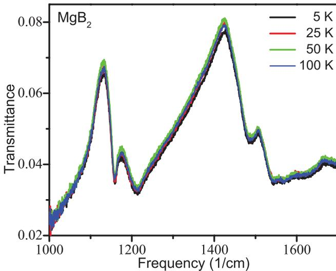
FIG. 7. (Color online) Experimental transmittance spectra around several EOT peaks on a  $\text{MgB}_2$  film in the mid-infrared regime. The film thickness is 50 nm. The array of holes has a lattice constant of  $6 \mu\text{m}$  and a hole diameter of  $3 \mu\text{m}$ . Representative spectra are shown here, with temperatures at 5, 25, 50, and 100 K. These are nearly overlapping.
