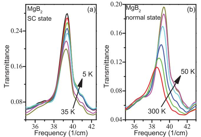
FIG. 6. (Color online) Experimental transmittance spectra around an EOT peak on a  $\text{MgB}_2$  film. The film thickness is 50 nm. The array of holes has a lattice constant of  $80 \mu\text{m}$  and a hole diameter of  $40 \mu\text{m}$ . (a) Spectra when  $\text{MgB}_2$  is in the SC state. Temperatures change from 5 to 35 K, with a step of 5 K. (b) Representative spectra when  $\text{MgB}_2$  is in the normal state. Temperatures change from 50 to 300 K, with a step of 50 K.
