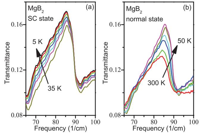
FIG. 5. (Color online) Experimental transmittance around an EOT peak of the  $\text{MgB}_2$  film. The film thickness is 50 nm. The array of holes has a lattice constant of  $50 \mu\text{m}$  and a hole diameter of  $25 \mu\text{m}$ . (a) Transmission spectra when  $\text{MgB}_2$  is in the SC state. Temperatures change from 5 to 35 K, with a step of 5 K. (b) Representative spectra when  $\text{MgB}_2$  is in the normal state. Temperatures change from 50 to 300 K, with a step of 50 K.
