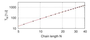
FIG. 3. (Color online) The SWAP operation time  $T_N$  versus the chain length N: the red continuous line is  $(N - 1)^2$  while the black dots are the lengths for which we numerically verified this scaling with a fidelity  $F > 1 - 10^{-4}$ .
