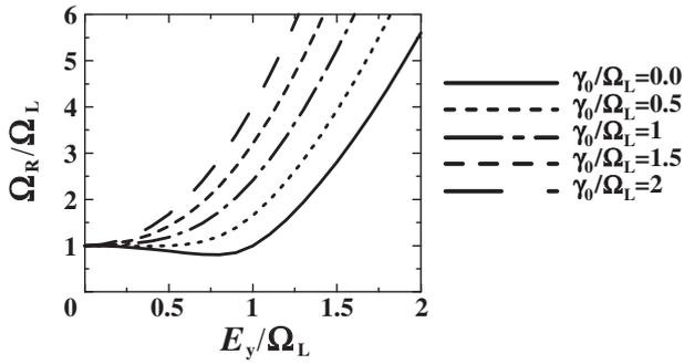
**Fig. 2.** The Rabi frequency  $\Omega_R$  needed for realizing a dark state, as a function of the detuning  $E_y$  and  $\gamma_0$ . Here,  $E_x = 0$ ,  $\gamma_{21} = 0$ ,  $t_0 = 0$ , and  $\Gamma_1 = \Gamma_2 = \Gamma_3$ . These are solutions of  $\rho_{33} = 0$  in eq. (9).
