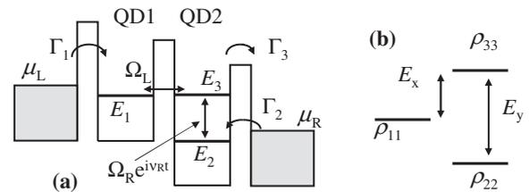
**Fig. 1.** (a) A three-level system in double QDs (DQDs). A bias voltage is applied between the left and right electrodes. (b) A density matrix for the three level. We define  $E_x \equiv E_3 - E_1$  and the detuning  $E_y \equiv E_3 - E_2 - \nu_R$ . The dark state is a state with  $\rho_{33} = 0$ .
