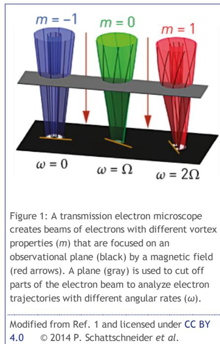
Figure 1: A transmission electron microscope creates beams of electrons with different vortex properties ( $m$ ) that are focused on an observational plane (black) by a magnetic field (red arrows). A plane (gray) is used to cut off parts of the electron beam to analyze electron trajectories with different angular rates ( $\omega$ ).
