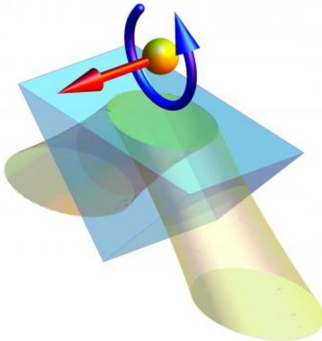
Transverse force and torque on a particle in evanescent field generated from a total internal reflection in a glass prism. These reveal the presence of the transverse momentum and spin in the evanescent wave above the prism. Credit: RIKEN
