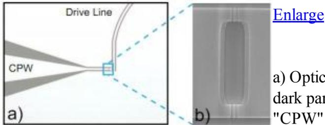
a) Optical micrograph of the device. Light parts are Al while dark parts are the Si substrate. The output line is labeled "CPW" and the drive line enters from the top. Both lines converge near the SQUID. b) A scanning-electron micrograph of the SQUID. Image credit:
