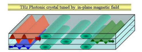
The array of green cylinders inside the sample, forming a socalled photonic crystal, span the width of the sample. These cylinders contain a magnetic field, and act somewhat similarly to bumpers in a pinball machine, scattering the incident electromagnetic waves, shown in red. Only red waves with certain frequencies can propagate through the crystal, resulting in the outgoing transmitted wave shown in green. The rest bounce back, shown as the reflected blue waves.
