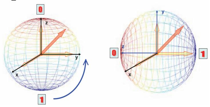
This rotation can be realized by setting  $\Phi_x = 0$  and  $n_{\rm C} = \frac{1}{2}$  with an evolution time  $t_x = \frac{\hbar \pi}{4 E_{\perp}^0}$ .
