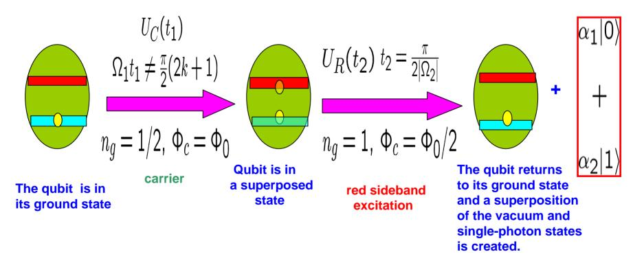
When the red sideband excitation satisfies the condition  $t_2 = \pi/2|\Omega_2|$ , it creates a superposition of the vacuum and single photon states.
