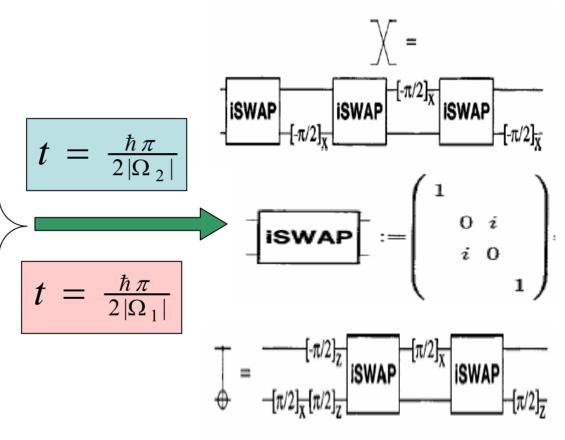
Quantum tomography can be implemented via an ISWAP gate, even if only one qubit measurement can be performed at a time.
