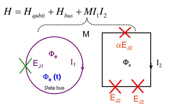
The circuit with an LC data bus models the Delft circuit in Nature (2004), which does not work at the optimal point for a TDMF to control the coupling between the qubit and the data bus.
