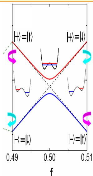
$$H_{0} = \frac{\hbar}{2} \left[ \omega_{1} \sigma_{z}^{(1)} + \omega_{2} \sigma_{z}^{(2)} \right] + \left[ g \sigma_{+}^{(1)} \sigma_{-}^{(2)} + \text{H.c.} \right]$$
